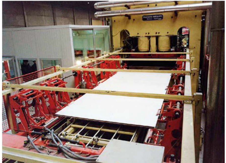
A press line working optimally would not be able to reduce or remove defects caused by inadequate storage or rough boards.
